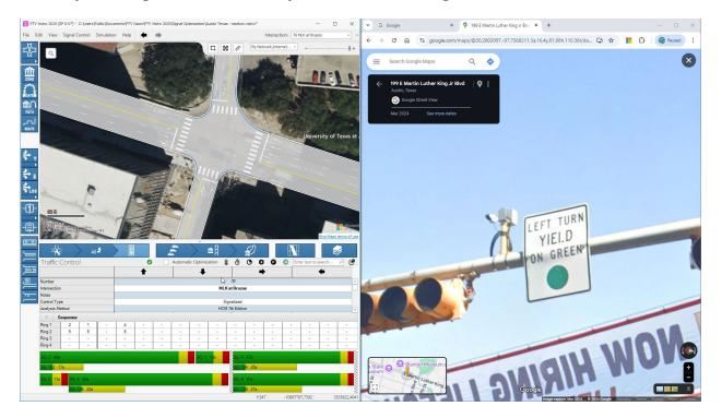
Vistro now features a visualization of turning movements and lane group turns, simplifying the modeling of complex intersections with over five legs. This tool provides clear path arrows to confirm lane configurations, ensuring more accurate volume and lane setup. Correct lane configurations enhance simulation accuracy in PTV Vissim and streamline detailed intersection modeling, improving overall project precision and efficiency.
