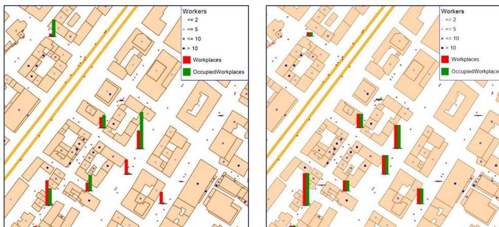
Figure 11: Doubly-constraint: In the traditional approach (left-hand chart), the target destination traffic is never achieved exactly; the number of employees at the place of work does not correspond to the number of jobs. With the methodology used by Visum, on the other hand (right-hand chart), the target figure is hit exactly.
